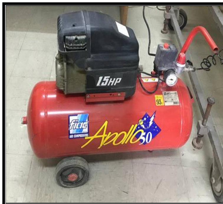
Figure(2.4): Air compressor
