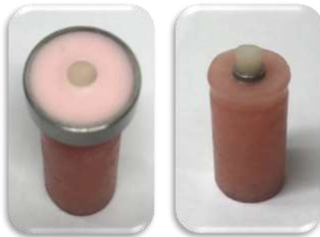
Figure 2.11: Cementation procedure over the titanium disc.
