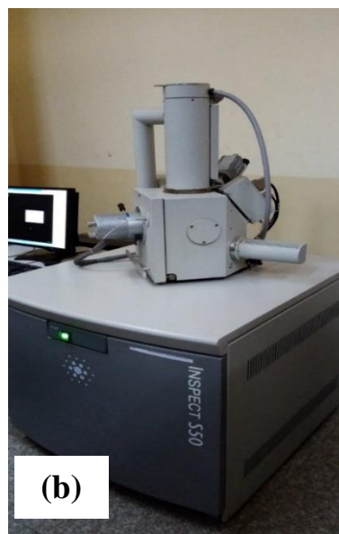
Figure 2.11: Specimens Surface Observations: a) Optical microscope type Lomo TM , b) SEM-EDS device type Inspect TM .
