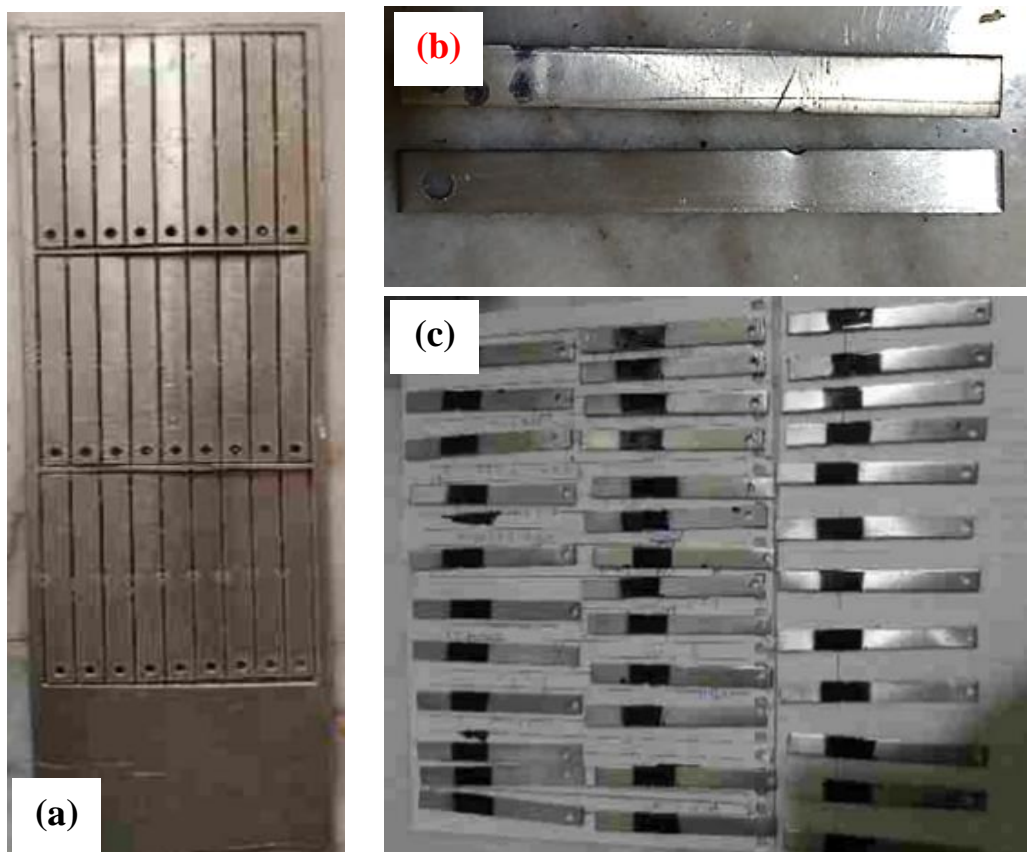
Figure 2.5: Steps of specimen's preparation for the fatigue test: a) after cutting with water, b) after polishing process and c) after coating the working area with black paint.
