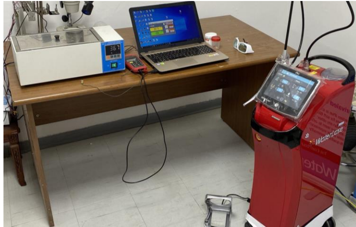
Figure (2-10) show the set-up for measuring temperature rise by Er:Cr:YSGG Laser ( consist of water-path and thermometer connected to a computer).
