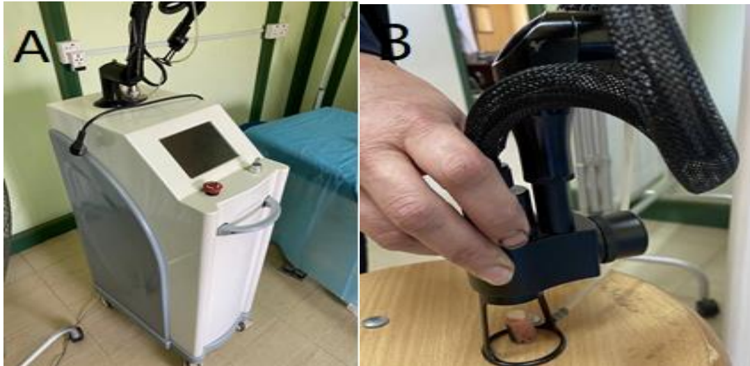
Figure (2-10) a) Fractional CO 2 laser, b) position of sample during lasing.
