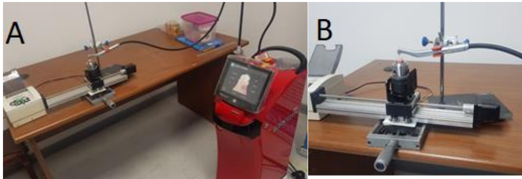
Figure (2-6) A) The set-up of the application of Er:Cr:YSGG laser with the CNC machine, B) The CNC Machine.
