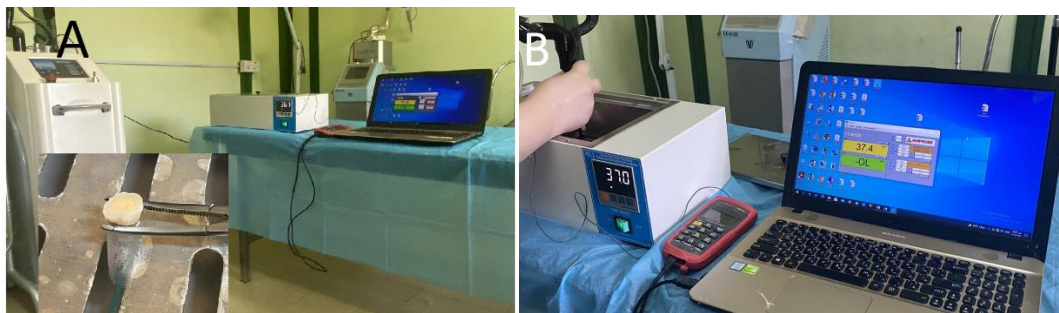
Figure (2-11) Set-up for measuring temperature with Fractional CO 2 Laser.
