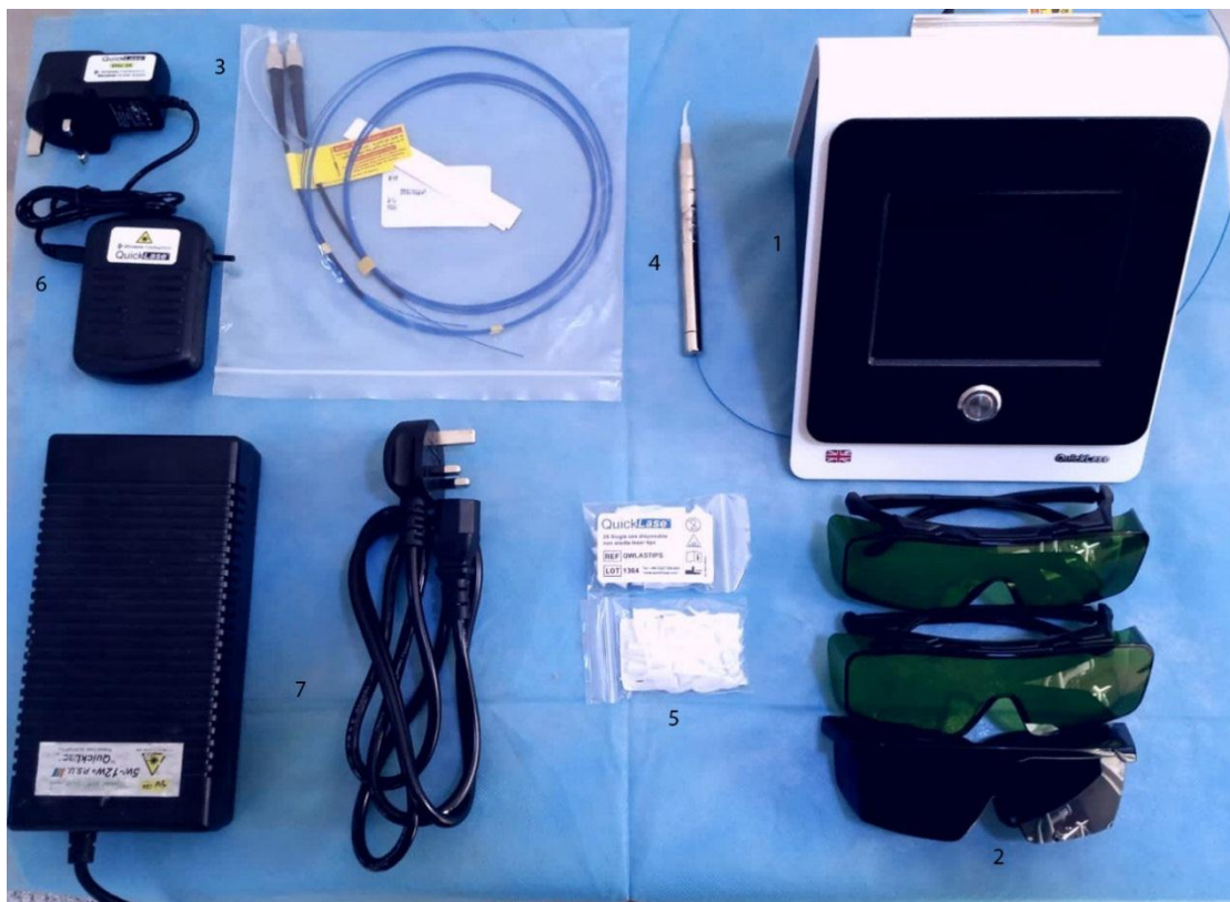
Figure (2-4): Components of diode laser device (QuickLase dentalase)
