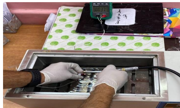
Figure (2.3): Thermocouples device to measurement heat temperature in the tooth during laser irradiation for Er.Cr:YSGG laser.
