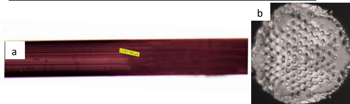
Fig.(3.6) Microscope image show a)length of infiltration region in PCF b) cross section of agarose infiltration in PCF ( AI-PCF)
