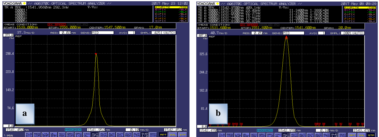
Fig.(3.21)a) Wavelength peak of PCFI before coating. b) The shift in Wavelength peak of PCFI after coating is about 1.014 nm
