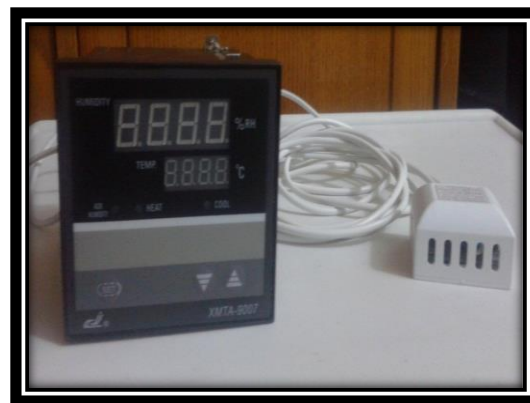
Fig. (2.15) Temperature and Humidity Controller
