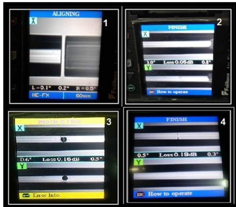
Fig.(3.1): The splicing process and the loss obtained in (dB)
