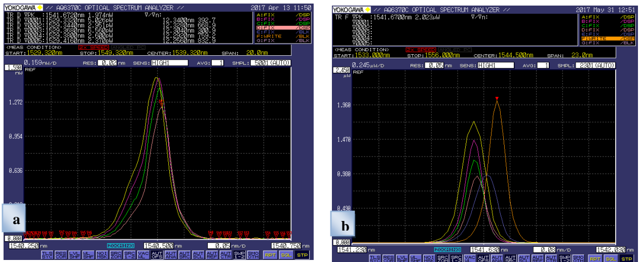
Fig. (3.27) OSA Graphics peaks shift of AC-PCFI(A) with respect humidity. b) OSA Graphics peaks shift of AC-PCFI(B) with respect humidity
