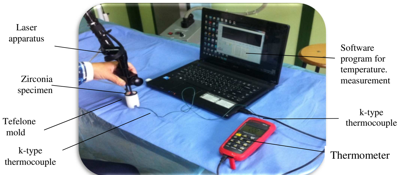
Figure (2-12) Temperature Measuring during laser irradiation
