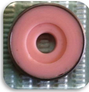
Figure (2-11) Silicone mold with a central opening for molding the resin cement
