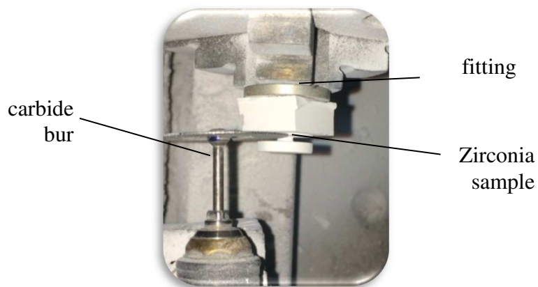
Figure(2-5) cutting with a carbide bur
