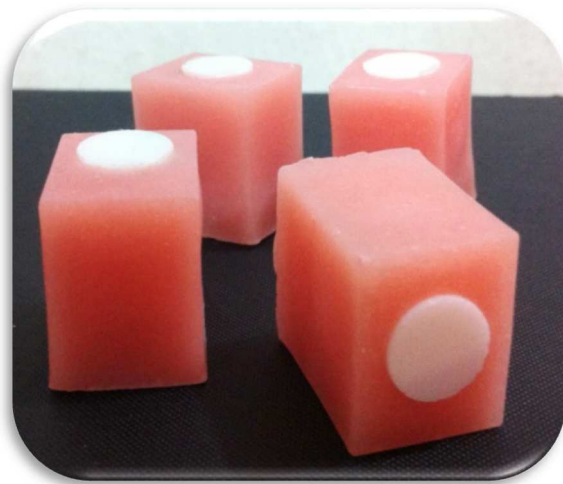
Figure (2-13) Acrylic block of zirconia disc
