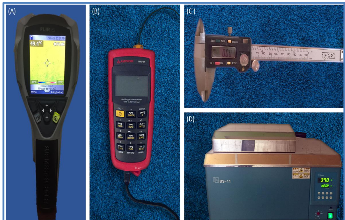
Figure 2-5: Some of equipment used in the study. (A) Thermal camera, (B) Thermometer, (C) Vernier caliper (D) Water bath
