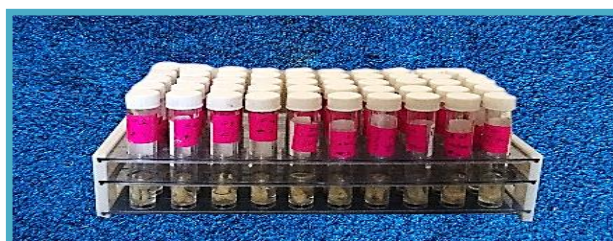
Figure 2-6: Sample of teeth stored in 4°C distilled water containing 0.1% thymol
