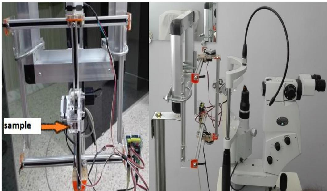
**Figure 2.4** Two dimensions Computer Numerical Control (CNC) work station
