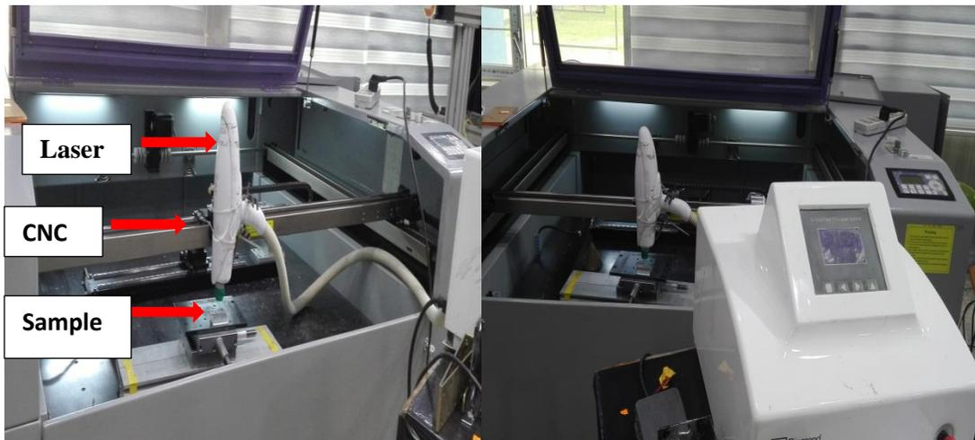
**Figure 2.5** Diamond Q-Switched Nd: YAG laser fixed on the CO<sub>2</sub> laser CNC work station
