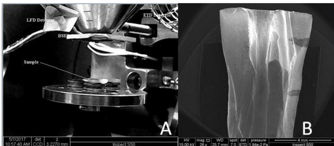
(Figure 2-17) **A:** Specimen fixed on the aluminum stub inside SEM device after gold metallized. **B:** Specimen at magnifying power 26x.
