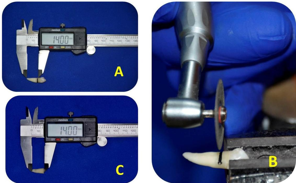
**Figure (2-2) A:** sample length determination, **B:** sectioning of the sample, **C:** root sample after sectioning.
