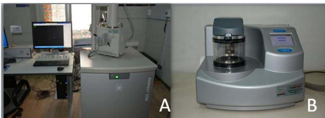
**(Figure 2-16) A:** SEM (Inspect S50, Czech Republic). **B:** Vacuum and sputter coater.
