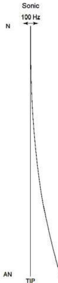
**Figure (1-2):** Oscillation pattern of sonically activated instruments. N represents the minimum oscillation while AN represents the maximum oscillation of the amplitude [47].
