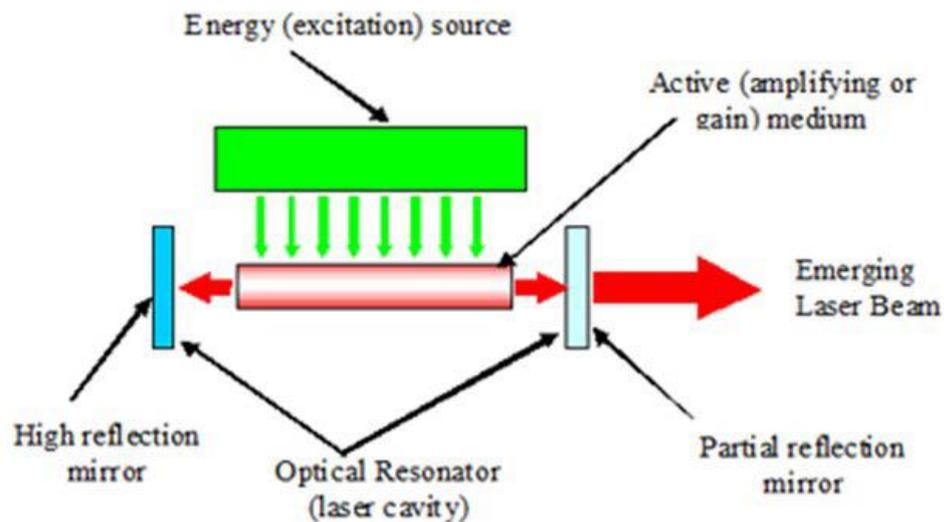
(Figure 1-10) Laser components [77].
