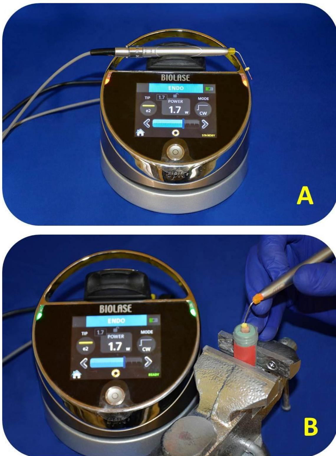
(Figure 2-14) A: Diode laser apparatus, Biolase, with endodontic fiber tip.
