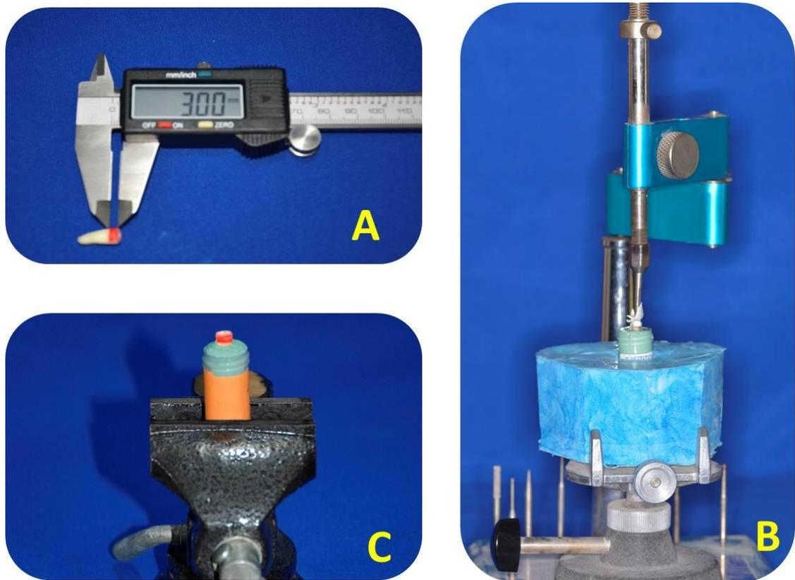
**Figure (2-5): A:** A line 3mm away from the coronal margin is drawn to mark the level of embedding in silicon-filled plastic tube. **B:** Inserting the sample in the silicon-filled plastic tube with the aid of surveyor. **C:** Mounting of the tube on the bench vice.
