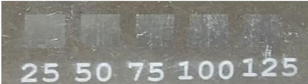
**Figure (3-22): Al 3003 treated by laser colorizing parameters
