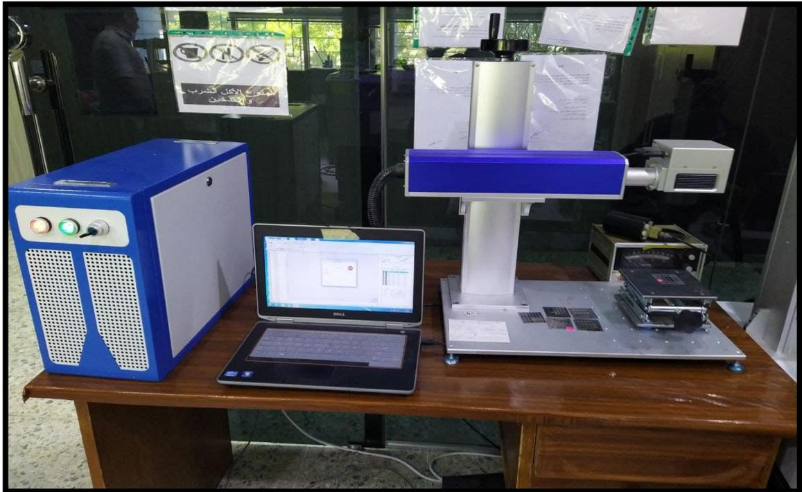
**Figure (2-1): Microsecond fiber laser.**
