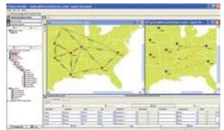
*Multiple views of the optical network in MetroWAND. Physical layer topology view and traffic demand view.*
