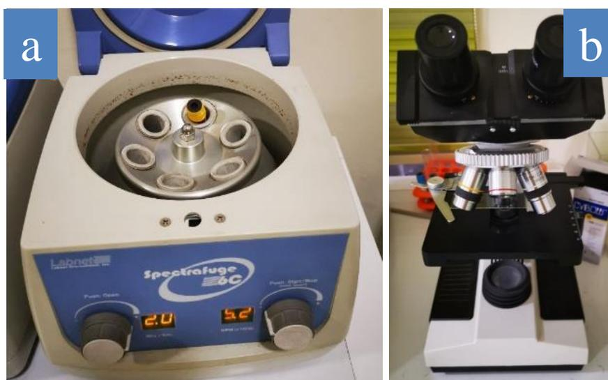
**Figure C.1:** Laboratory devices (a) Centrifuge (b) Optical Microscope
