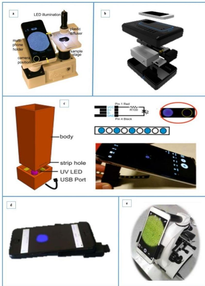
**Figure 1.15:** Biochemical applications of smartphone adapter (a) Transmission light microscope based on smartphone, [59], by Skandarajah, et al. under the Creative Commons license. (b) Smartphone-based adapter, [61], by You, et al. © copyright 2017 American
