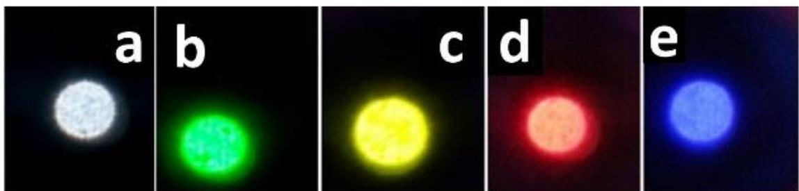
**Figure 3.3:** Images of the smartphone adapter using white LED as illumination source (a) without the emission filter (b) with the emission filter FB530-10 (c) with the emission filter FB580-10 (d) with the emission filter FB640-10 (e) with the emission filter FB430-10
