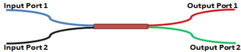
**Fig. (1.3):** Schematic Diagram of Fiber Output Coupler [57].
