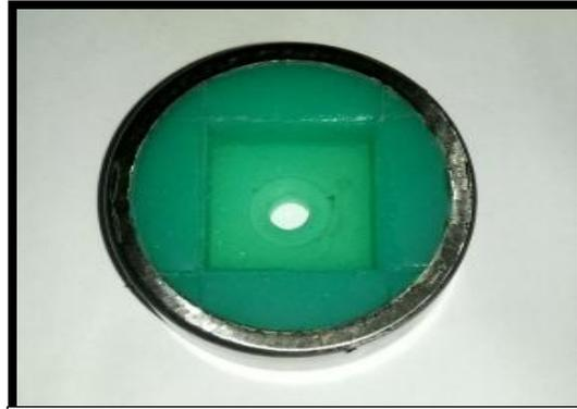
**Figure (2-10):** Silicone mold with central opening for resin cement molding
