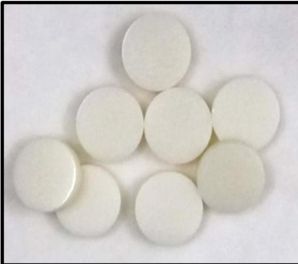
**Figure (2-4):** CAD-CAM milled zirconia samples
