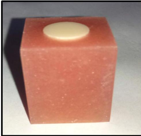
**Figure (2-17):** Acrylic blocks with zircons discs
