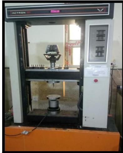
**Figure (2-23):** Universal testing machine
