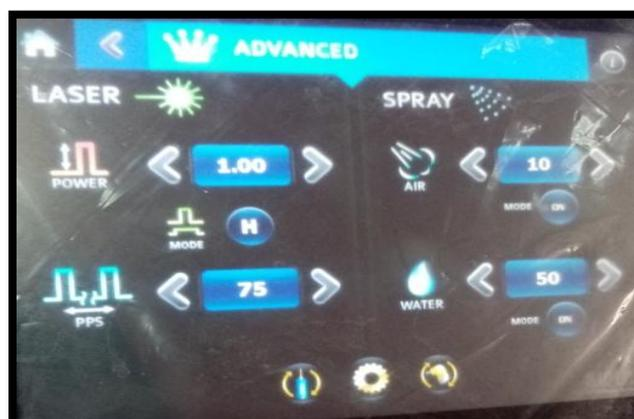
**Figure (2-11):** Control panel of the Er,Cr:YSGG laser device
