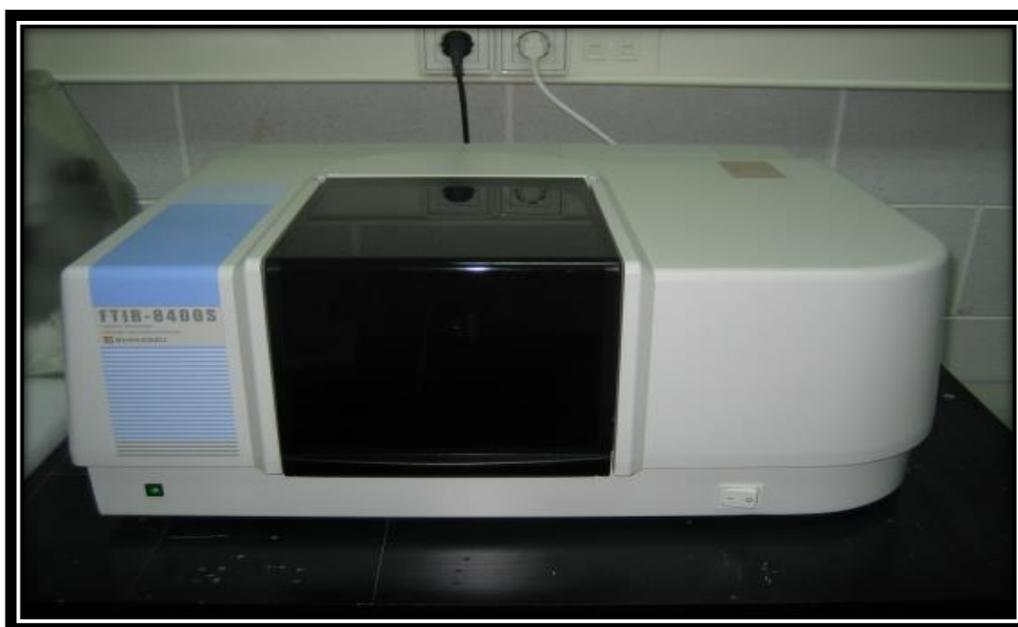
**Figure (2.8): Fourier transformation infrared Spectrometer.**
