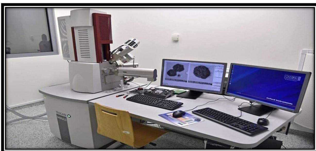
**Figure (2.10): Field Emission Scanning Electron Microscope**
