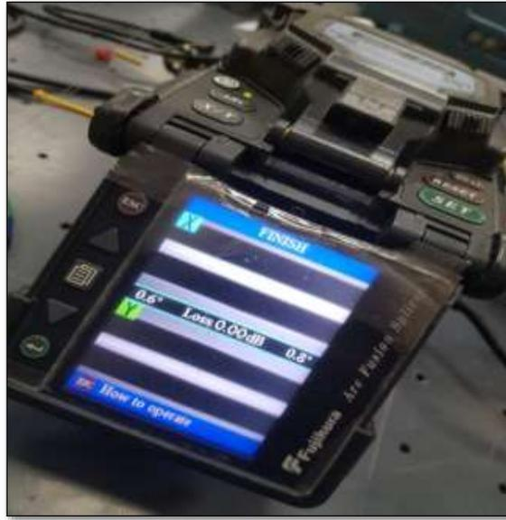
Fig. (2.5): photograph of (FSM-60S) fusion splicer
