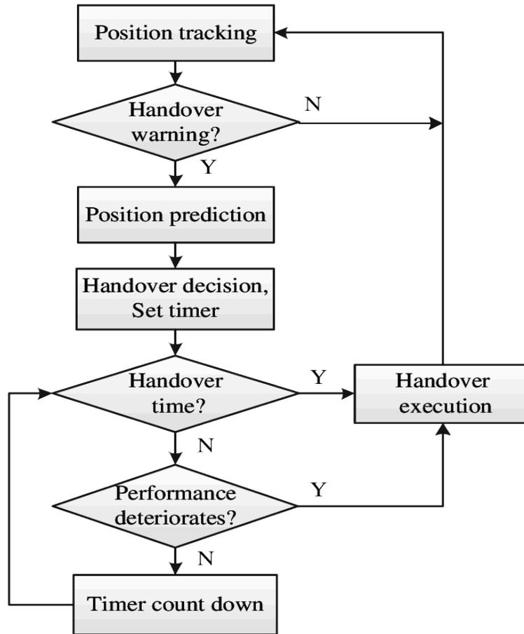
Fig. 2.3.: The signalling flow chart of traditional mobile network
