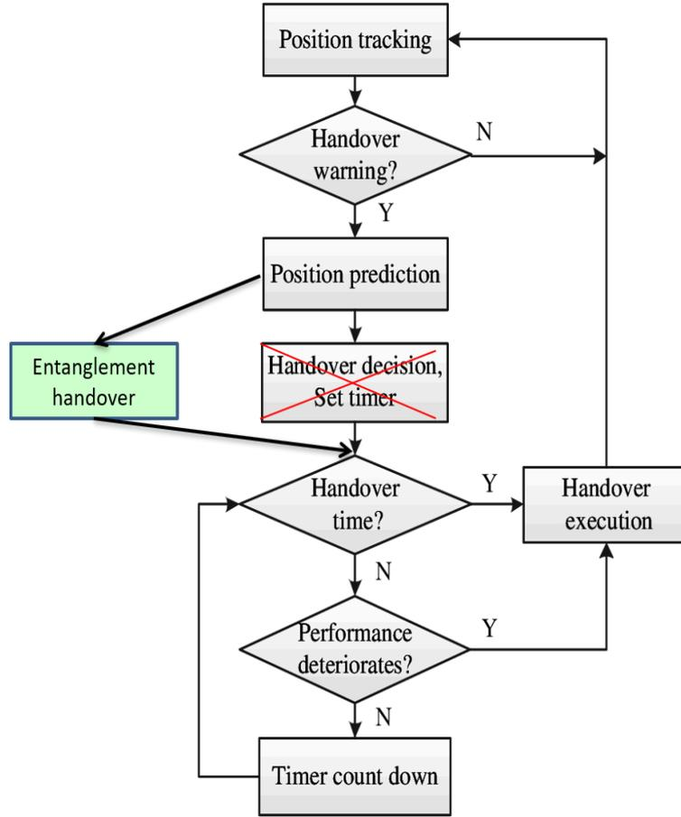
Fig. 2.4.: The signalling flow chart of entanglement based mobile network
