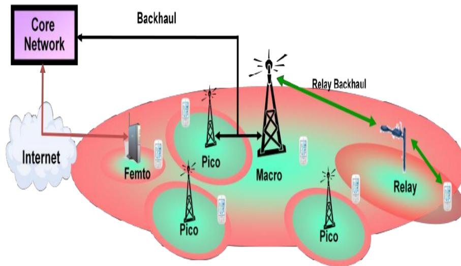
Fig. 1.5.: Heterogeneous network architecture [10].
