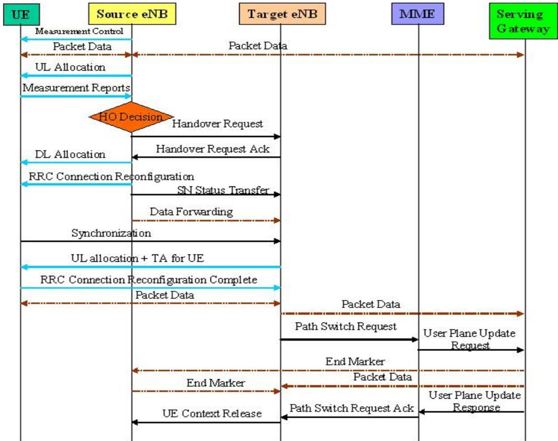
Fig. 2.2.: The signalling procedure of traditional mobile network handover.
