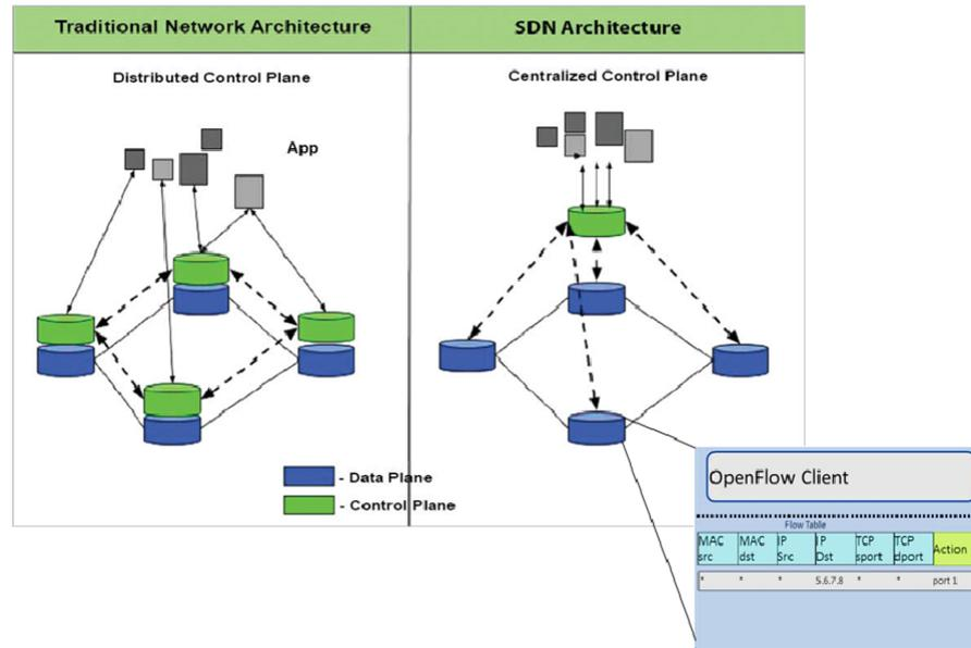
Fig. 1.6.: Comparison between SDN and traditional network architecture [34].
