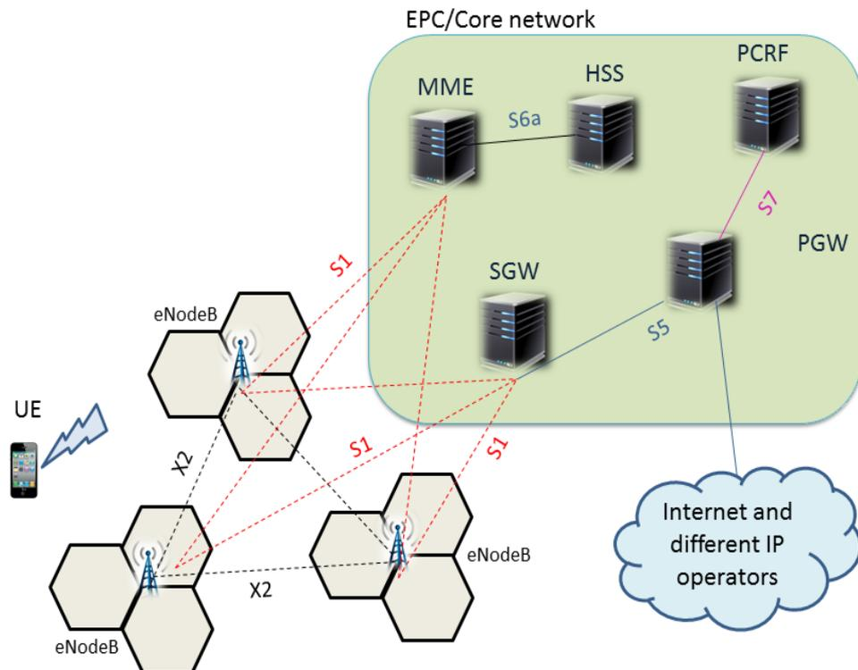
Fig. 1.2.: LTE E-UTRAN architecture [13]. It presents three main sections of LTE: EPC, E-UTRAN and UE. E-UTRAN with many eNodeBs, EPC contains PGW, SGW, PCRF, HSS and MME units.
