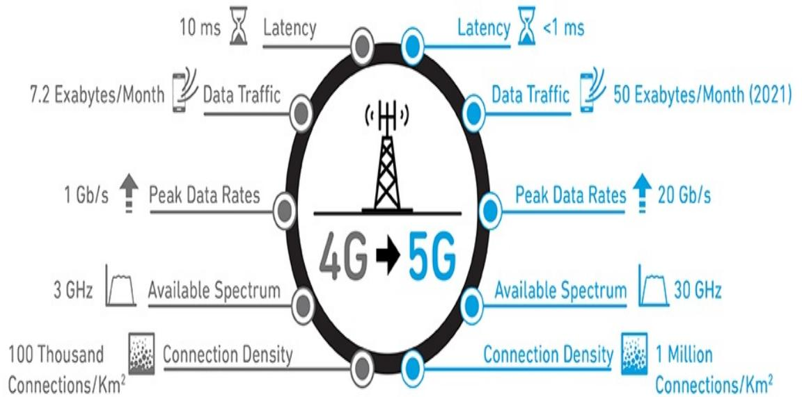
Fig. 1.3.: Comparison of 4G and 5G requirements [25].
