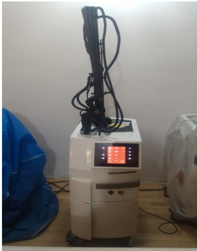
Figure (2-2) Er: YAG laser system 2940 nm
