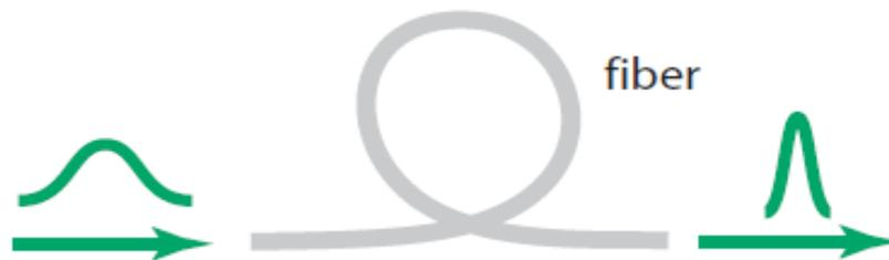
**Fig. 1.21** A schematic configuration for high order soliton compression [62].
