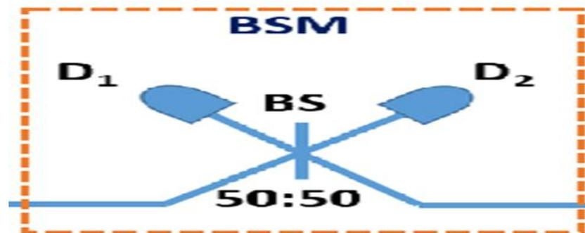
**Fig. 1.9: Bell State Measurement BSM.** The bar is 50:50 beam splitter BS,  $D_1$  and  $D_2$  are detectors.
