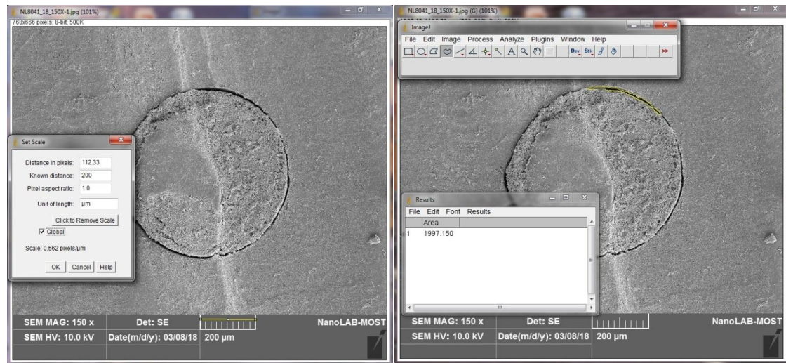
Figure (2-14): Measurement of the gap at x150 with the aid of Image J software program.
