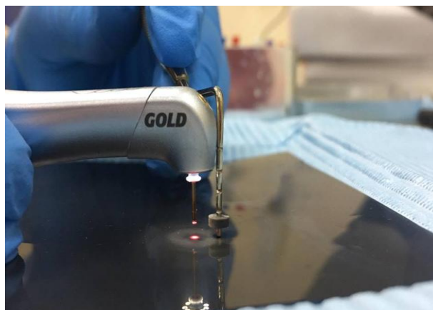
Figure(2-18): A photograph shows the establishment of 1mm spot size diameter.
