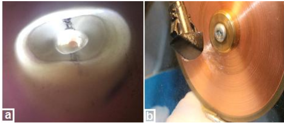
Figure (2-12): Sectioning of tooth to prepare it for SEM evaluation (a) demarcation of lines that divided the root into two equal halves (b) tooth sectioning with diamond warfaring blade.
