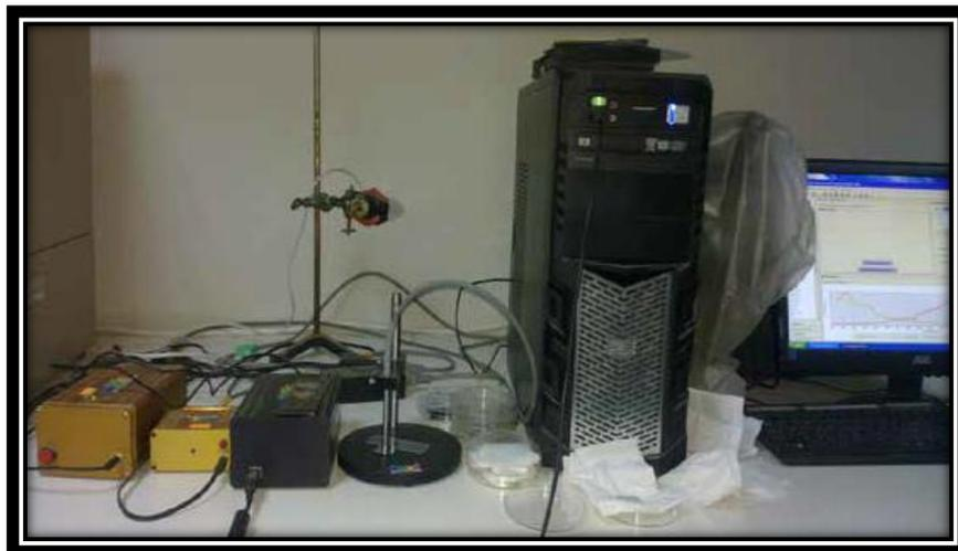
**Fig. (2.12): Thin Film Measurement System Model Epp 2000.**
