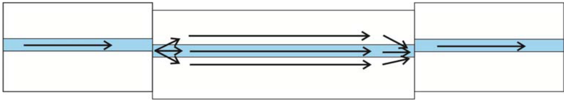
Figure (1.6): a schematic profile of core-offset fiber Mach-Zehnder interferometer [33].
