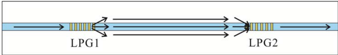
Figure (1.7): LPG based Mach-Zehnder interferometer (LPGMZI) [31].
